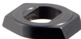
Front base, for pivot mount, to be installed in the running rail, available in the heights 5,0 mm (bottom open) and 6,0 mm (bottom closed) for rib width of 14 mm
