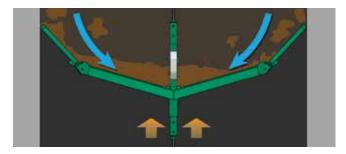
On the return stroke of the scraper, toggling blades pivot upwards to avoid bringing the manure back to the starting point. The ends fold towards the inside of the alley to leave sufficient space alongside the rest area and to avoid disturbing the cows.
