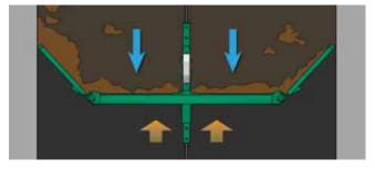
The draw bar rides in the groove for stable scraper operation even in the event the manure load is not distributed equally on each side of the scraper.
