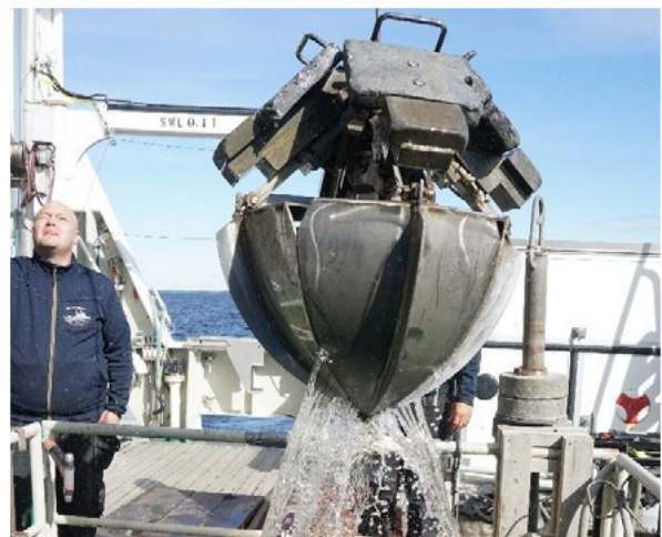
Sediment sampler, Orange Peel Bucket (OPB), being retrieved back on deck. (Photo by Geological Survey of Sweden)
