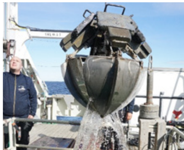
Sediment sampler, Oragne Peel Bucket (OPB), being retrieved back on deck. (Photo by Geological Survey of Sweden)
