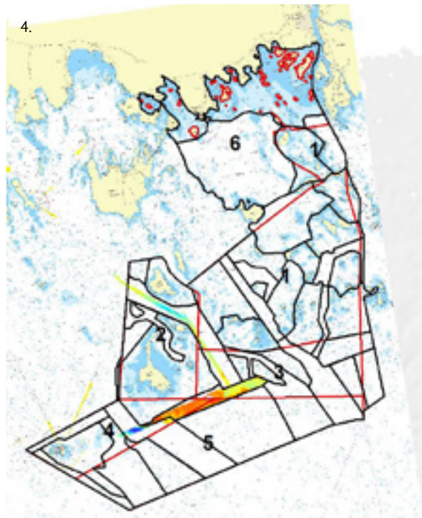
4. A first draft of our adapted survey plan (black lines), which also includes a small overlap into Finland to ensure seamless maps between our two countries - the oceans know no borders as we all know, but sometimes forget. Surveying in coastal areas with complex and partly unknown topography is very challenging for survey planning. We think we have gotten off with a good start though! Some areas are deep enough for S/V Ocean Surveyor, and the shallower areas Ugglan will take care of. Not all areas will be surveyed as time is limited. Which areas we will cover depends both on priorities (see numbers in the image and the red lines) prevailing winds and overall weather conditions during the next six weeks. We hope the fall storms will wait a bit longer since the outer areas are very exposed.
