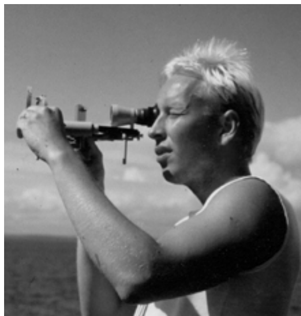
Positioning with sextant onboard the research vessel Geola in the late 1980's. (Photo by GTK)
