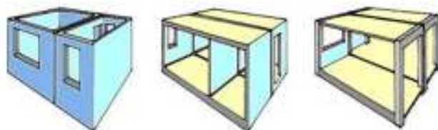
Figure 3: Classification of box unit systems
